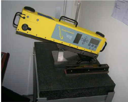
This is a calibrated inclinometer ( SunSight Classic AAT )
