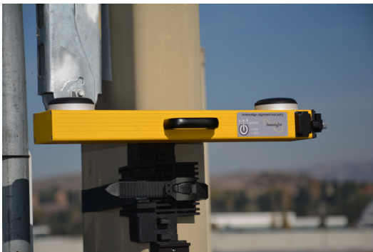
This is a calibrated azimuth alignment tool ( New SunSight AAT-30 )
