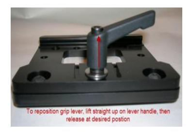
At no time should any effort be made to remove the 3mm grip lever retaining screw unless instructed to do so by an authorized agent of Sunsight Instruments. Removal of this screw can lead to grip lever failure.
